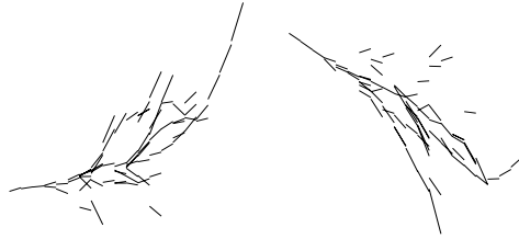
Fig. 9.4. xz projection (left) and yz projection (right) of a reconstructed shower generated by a 6 GeV electron interacting in the \sim 3.3 X_0 ECC exposed at DESY. Each segment corresponds to a base-track associated with the reconstructed electromagnetic shower.
