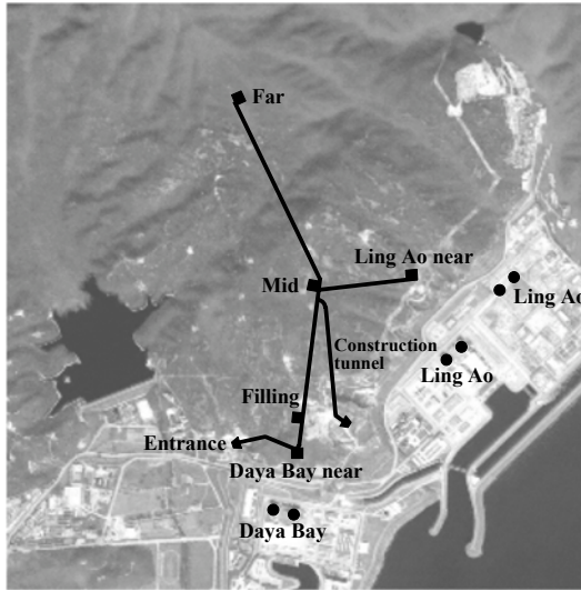
Fig. 13.2. Layout of tunnels and underground experimental halls.
